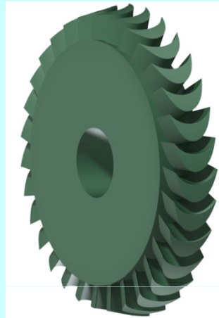
Meridional section of the baseline single-stage axial ORC turbine (left) and 3D model of the rotor (right)
